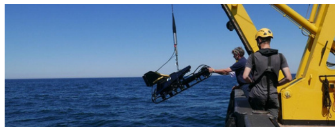
Figure 2: the Video Plankton Recorder (VPR) ready for deployment behind the Research Vessel (RV) Simon Stevin.
